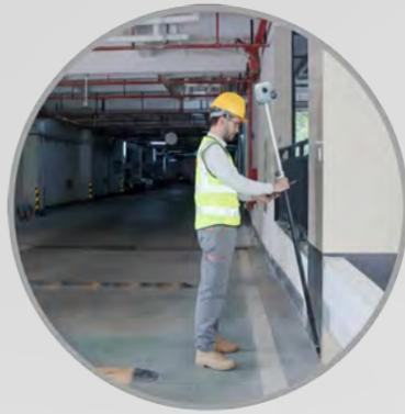
ME system is capable to maintain 5 cm accuracy for a few minutes when GNSS satellite signals are out-of-reach, the solution status will change from "fixed" to "Mixed Solution".
