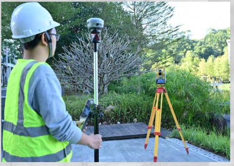
RTK GO 2025 now enable surveors to work GNSS receiver and Robotic Total station jointly. When a GNSS receiver being installed onto prism pole, Robotic total station can track prism with higher efficiency by using GNSS data, it greatly helps when you are working in complicated terrain and prism sometimes being blocked.
