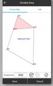
Select points to form a polygon, and directly identify the area division points for the surveyor to stake out. There is no more need for the user to guess a position to measure, and then to adjust.
