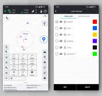
This feature allows you to draw the result map while completing point measurements.
