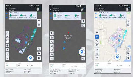
CAD Stakeout allows you to import CAD basemap and stakeout it, without inputting point coordinates one by one.
