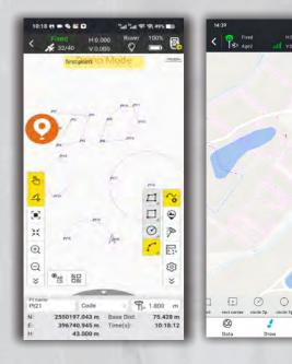
Select points to form a polygon, and directly identify the area division points for the surveyor to stake out. There is no more need for the user to guess a position to measure, and then to adjust.
