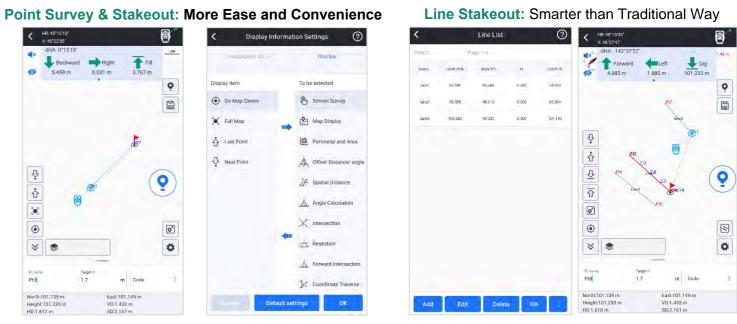
With graphic display, now it is easy to you to observe the relation between occupied point and target points. It will help you to make less mistakes when measuring many points.
