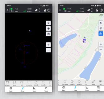
This feature enables CAD drawing capabilities, which were previously only possible on a PC. Now surveyors can edit CAD map on RTK controller or tablet or phones.
