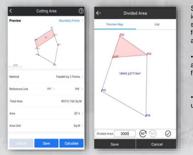
Select points to form a polygon, and directly identify the area division points for the surveyor to stake out. There is no more need for the user to guess a position to measure, and then to adjust.
