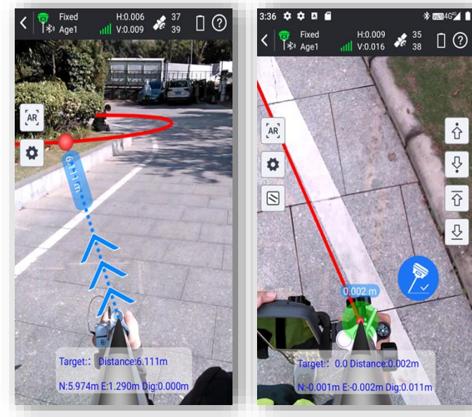
(This function only works with the receiver models that have downward-facing camera or dual-cameras)
