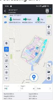
CAD Stakeout allows you to import **CAD basemap** and stakeout it, without input point coordinates one by one.
