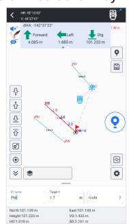
User is allowed to manually choose points from library, line will be formed by program automatically. Then user input interval distance, setout points will be calculated out and displayed on screen.
